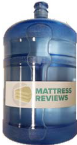
Figure 1: Reference Load 1. Plastic 5 gallon water cooler bottle. Size: 10.75" diameter, 19.5" height, 42.3 lb weight
