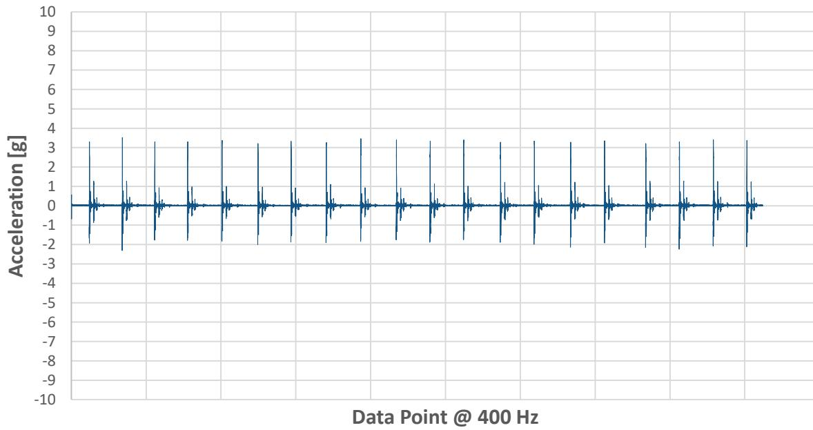
**Y Acceleration (Head to Toe) - Saatva**
