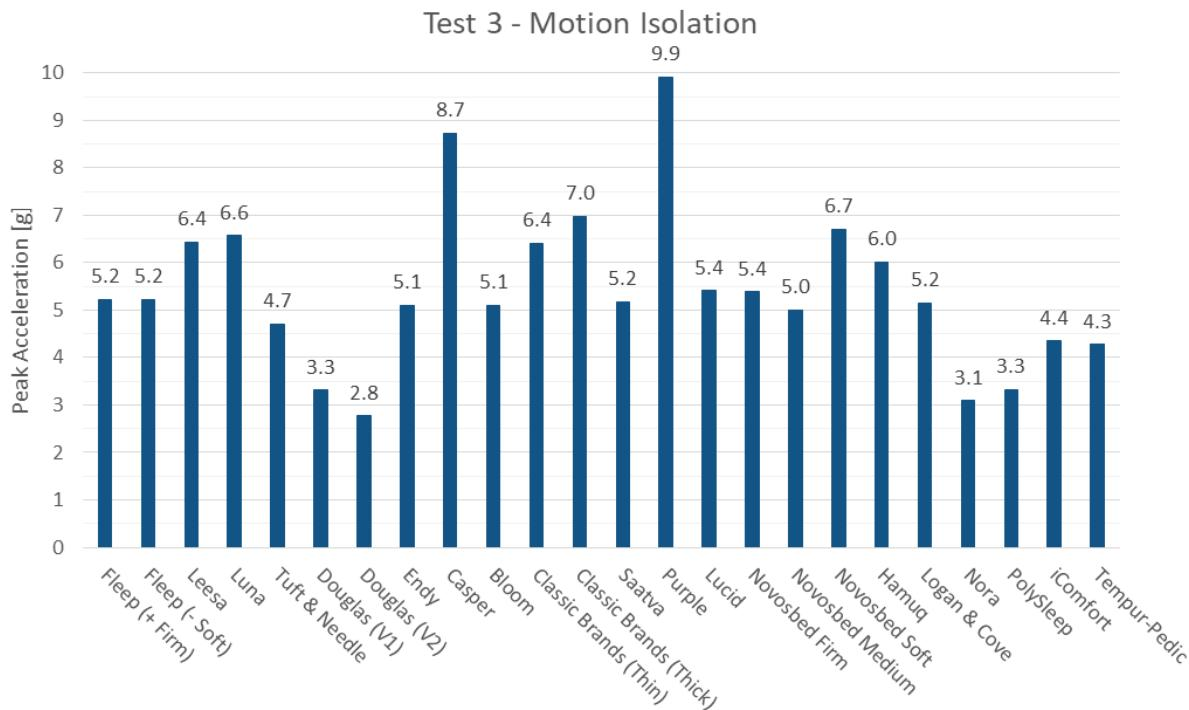
Figure 15: Peak Acceleration at one sleep point when Reference Load 2 is dropped on the other sleep point. Values shown are an average of 20 runs per mattress.\*
