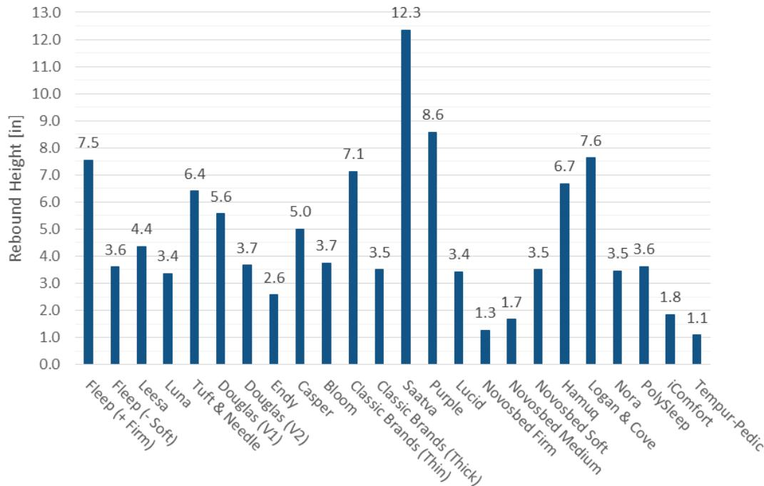
Figure 17: Rebound height of Reference Load 2 when dropped in the center of the mattress. Values shown are an average of 3 runs per mattress.
