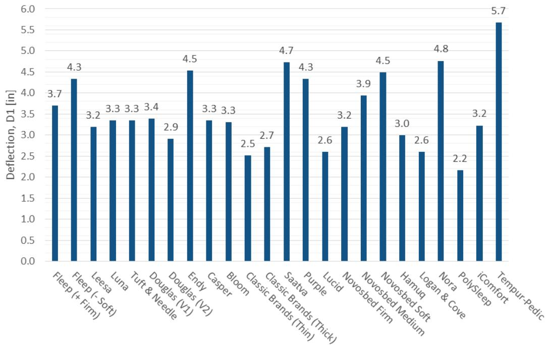
Figure 13: Test 2 – Mattress Firmness measuring how far Reference Load 1 deflects on the edge of the mattress. A higher number indicates larger deflection (or a softer mattress).
