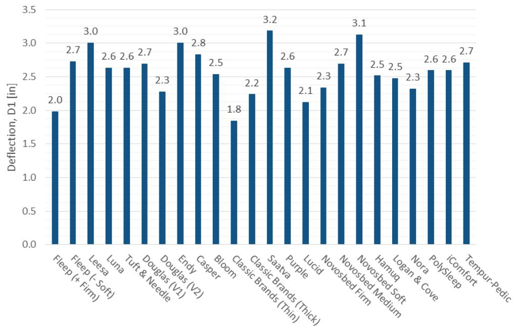
Figure 11: Test 1 – Mattress Firmness measuring how far Reference Load 1 deflects in the center of the mattress. A higher number indicates larger deflection (or a softer mattress).
